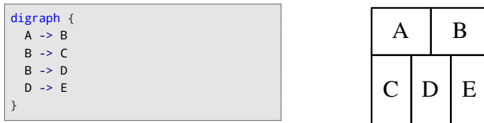
Figure 6.3: A simple digraph, rendered by patchwork . Note that patchwork ignores the edge relationships between nodes and simply partitions the canvas into one tile per node.
