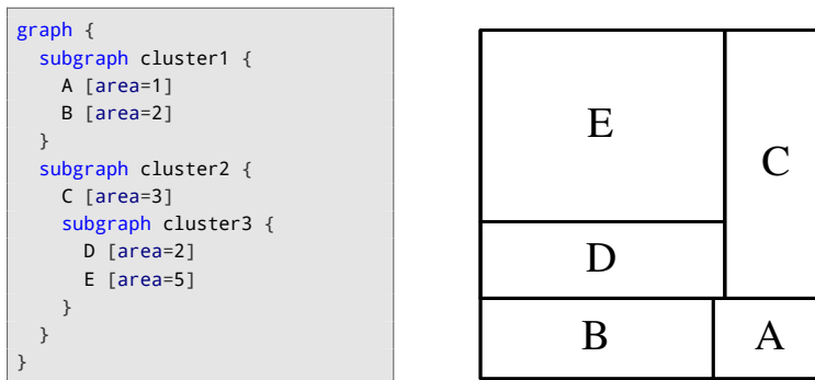
Figure 6.5: patchwork arranges the tiles on the treemap such that each cluster of nodes is grouped into a contiguous rectangle on the treemap.
